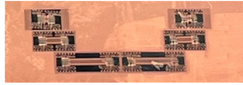
Fig. 3: The CPW structure connecting 6 pairs of chips with 3 different distances.
