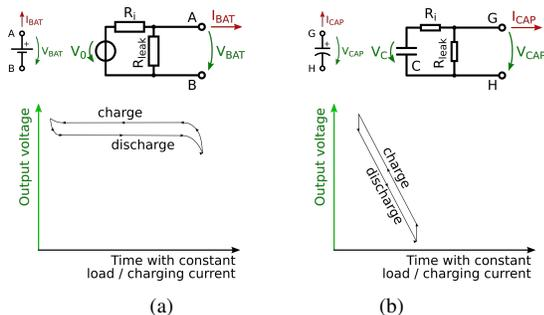
Fig. 2. Comparison of the charging and discharging curve of (a) Li-ion batteries and (b) super-capacitors. At the top the respective basic equivalent circuit is shown.
