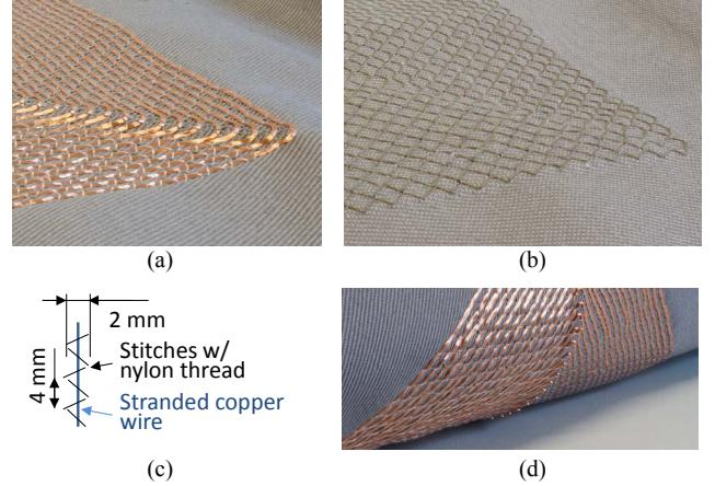
Fig. 2. (a) Embroidered stranded copper wire using nylon thread, (b) backside of the same cloth, (c) embroidery dimensions, and (d) photo of bent textile antenna.
