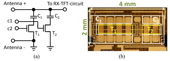
Fig. 9. Digital channel select circuit (a) schematic and (b) die photo. Transistor dimensions:  $T_1$  (W/L):  $8 \times 300 \mu\text{m} \times 5 \mu\text{m}$ ,  $T_2$ :  $4 \times 300 \mu\text{m} \times 5 \mu\text{m}$ . Capacitances:  $C_1 = 606 \text{ pF}$ ,  $C_2 = 303 \text{ pF}$ .
