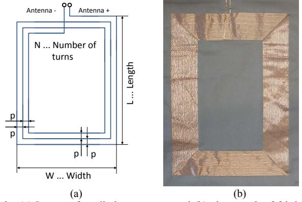
Fig. 3. (a) Layout of textile loop antenna and (b) photograph of fabricated antenna with  $N = 30$  and  $p = 2$  mm.
