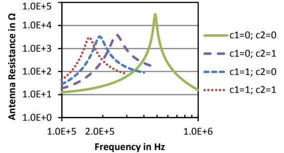
Fig. 10. Effect of the channel select TFT circuit and different digital input words *c1,c2* on the antenna resistance of antenna sample A30-2.
