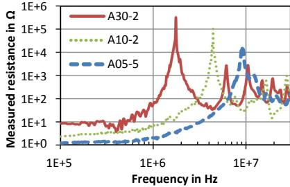
Fig. 4. Measured antenna resistances.
