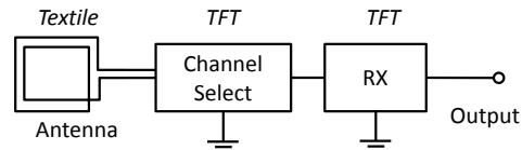
Fig. 1. System architecture of the target OOK-receiver (RX).
