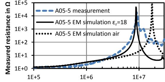
Fig. 6. Simulated antenna resistance of antenna A05-5.
