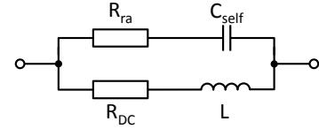
Fig. 7. Antenna model of lumped components.
