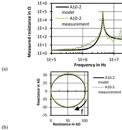
Fig. 8. Antenna sample A10-2. (a) Comparison of measured and modelled resistances in the frequency range from 100 kHz to 30 MHz. (b) Comparison of measured and modelled impedance in the frequency range from 100 kHz to 10 MHz.
