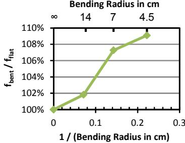
Fig. 5. Effect on  $f_c$  of bending antenna A10-2 along its “length”-axis.
